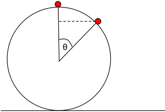
The sphere will fall a vertical distance  $R - R\cos\theta$  and so the speed at the point shown is found by energy conservation to be:
