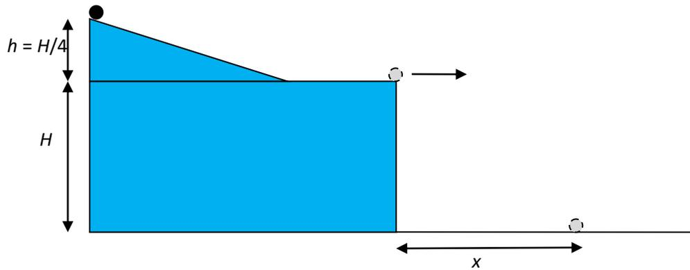
The ball will leave the rectangular block horizontally with speed  $v = \sqrt{2gh} = \sqrt{2g \frac{H}{4}} = \sqrt{\frac{gH}{2}}$ . The time to
